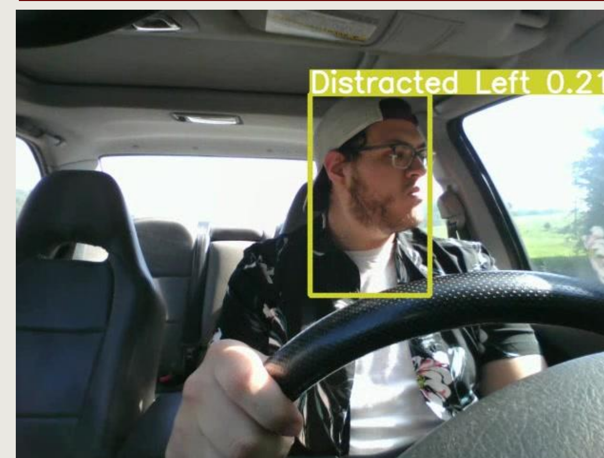
Image 1 shows the Distracted Driver model successfully detecting a driver, distracted by looking left with a 0.21 confidence level.
