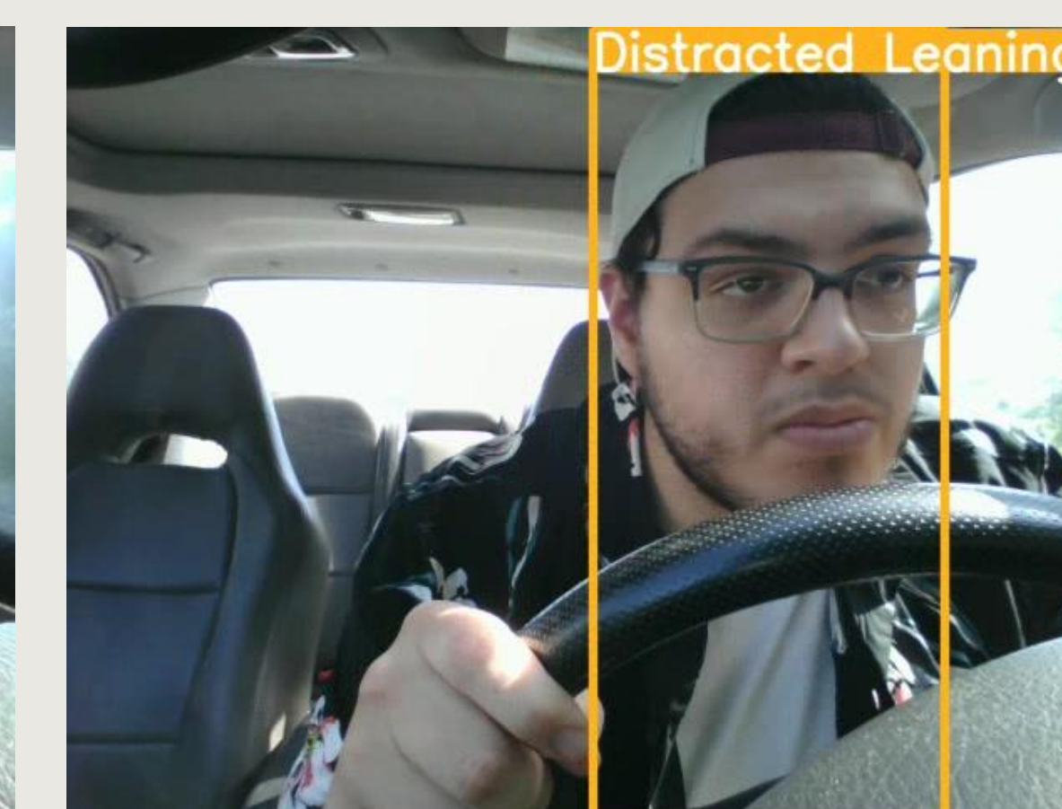
Image 7 shows the Distracted Driver model successfully detecting a driver, distracted by leaning forward with a 0.32 confidence level.
