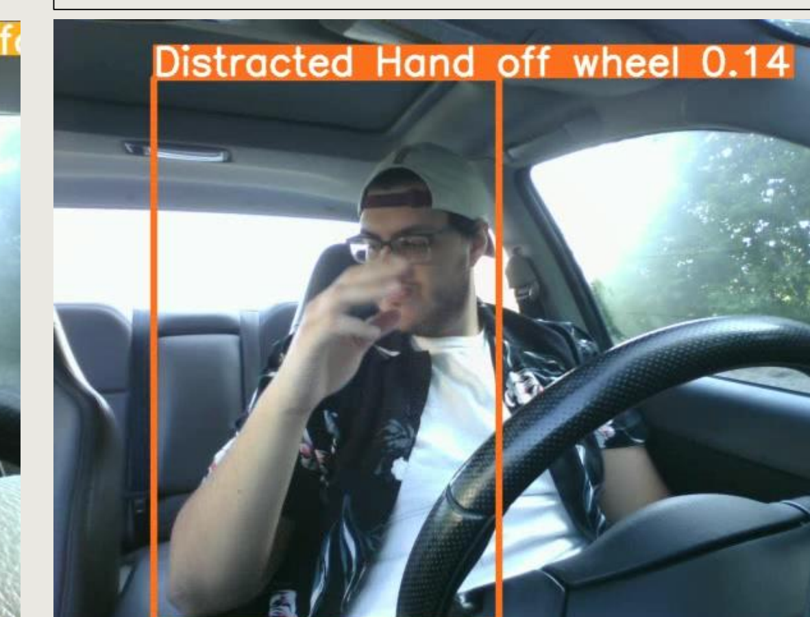
Image 8 shows the Distracted Driver model successfully detecting a driver, distracted by taking their hands off their wheel with a 0.14 confidence level.
