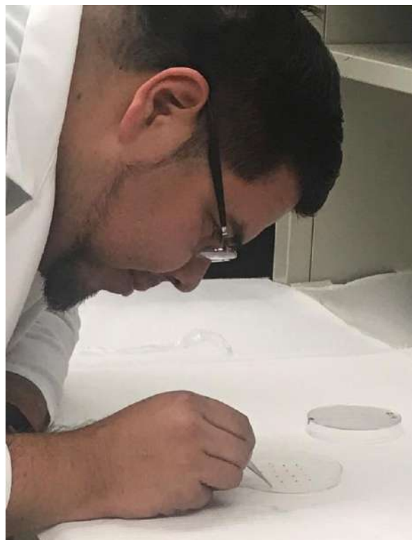
Samuel Ramirez is seen here, planting Palmer amaranth seeds on moistened filter paper in Petri plates.
